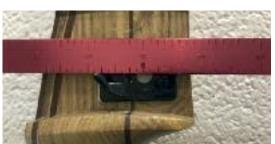
The bracing height is measured through the middle of the pressure button hole.
