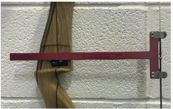
A bracing height gauge in use.
