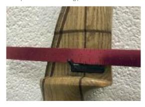
When checking the nocking point height, the bracing height gauge sits on the arrow rest
